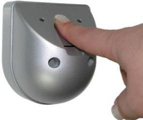
Place the finger onto the sensor.
